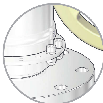
Horizontal and vertical movements stops by steps of 22.5°
